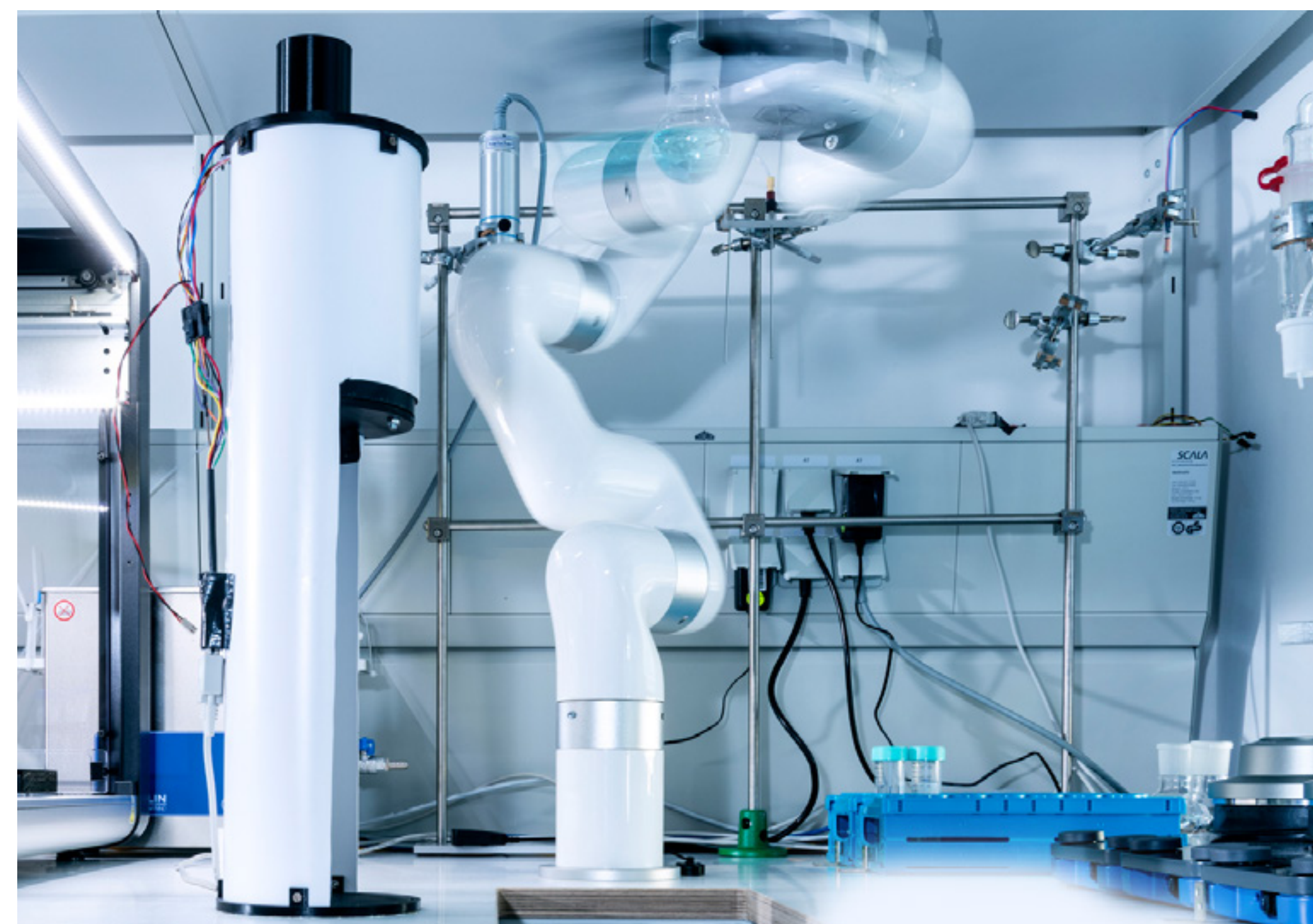
In the digitally controlled system, material synthesis, purification, and analysis take place with virtually no manual intervention.
