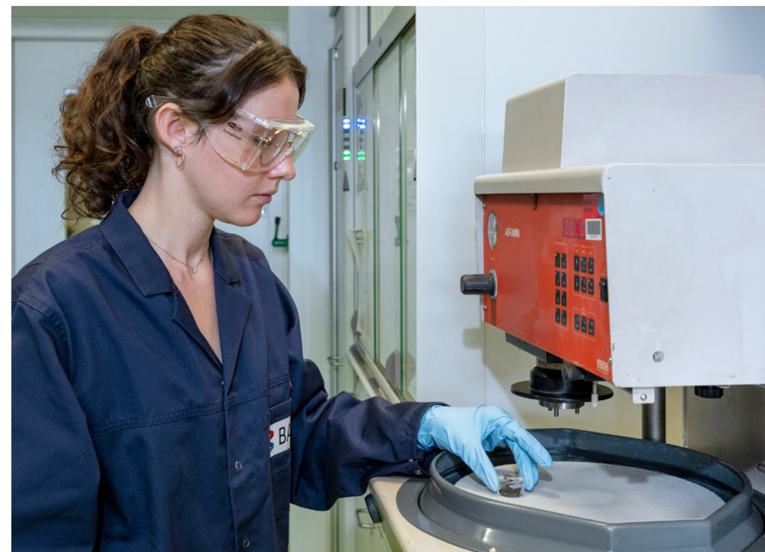
Iron samples of varying quality (r.), preparation of samples for microscopic examination (b.).
