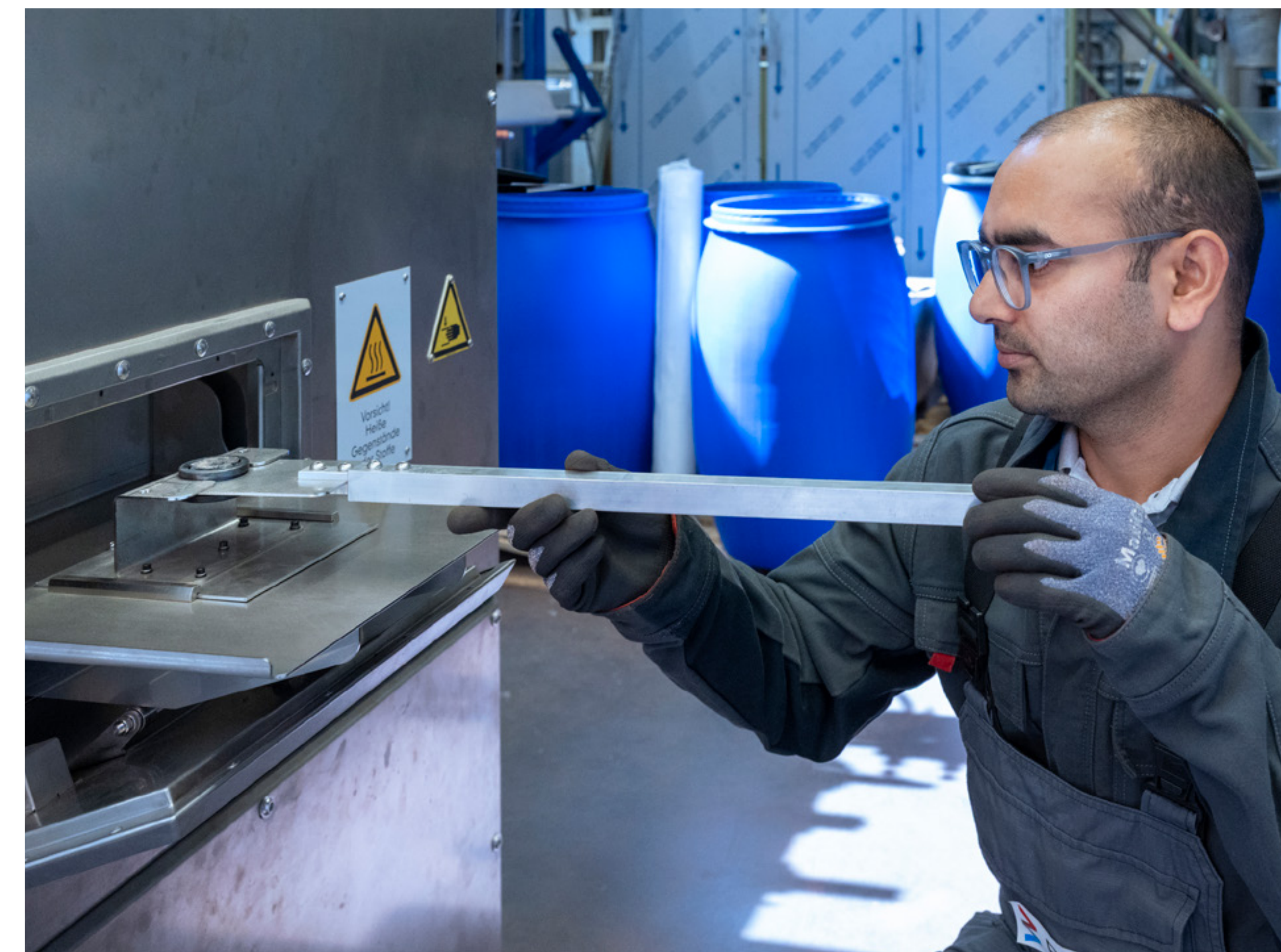
Analysis of the resulting slag using laser-induced plasma spectroscopy.
