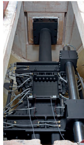
Intermediate-scale test stand integrated in column test furnace at BAM
