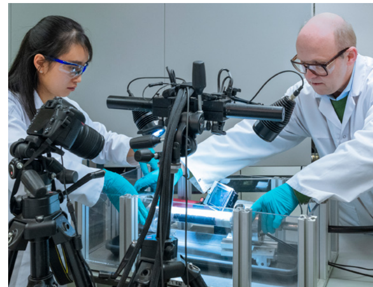
Deformations in the pipe are measured optically using high-resolution cameras.
